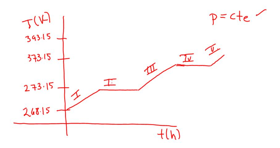
$$\Delta HI = N^{C}p(T_{Z}-T_{1})$$
